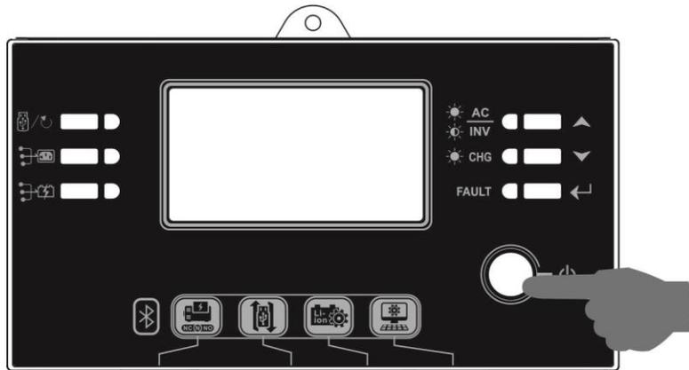
Once the unit has been properly installed and the batteries are connected well, simply press On/Off switch (located on the display panel) to turn on the unit.
