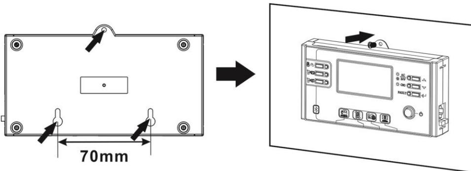
**Note:** Installation to the wall should be implemented with the proper screws. Refer chart for recommended spec of screws.
