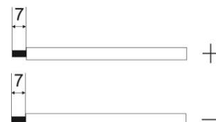
pole (-) of PV input connector. Screw two wires tightly in clockwise direction.
