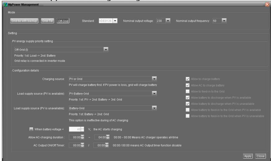
**PV energy supply priority setting:** 1<sup>st</sup> Load, 2<sup>nd</sup> Battery
