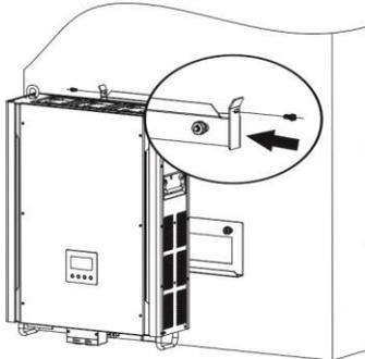
4. Check if the inverter is firmly secured.
