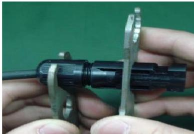
Step 4: Check correct polarity of connection cable from PV modules and PV input connectors. Then, connect positive pole (+) of connection cable to positive pole (+) of PV input connector. Connect negative pole (-) of connection cable to negative pole (-) of PV input connector.
