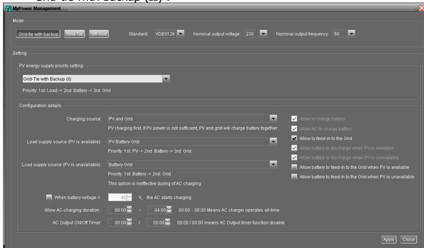
**PV energy supply priority setting:** 1<sup>st</sup> Load, 2<sup>nd</sup> Battery and 3<sup>rd</sup> Grid.
