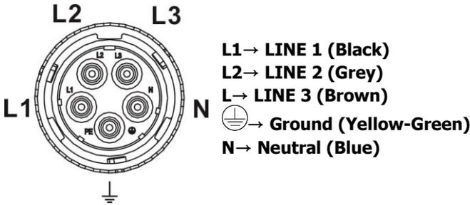
The reference tightening torque is 1.5-2.5 N.m.
